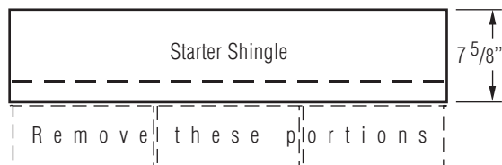
Figure 12-6: Make starter shingles that are 7 5 / 8 " in height.
